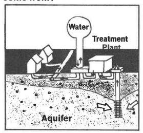
Lakemore's drinking water is pumped out of the ground from a well. This groundwater is pumped to the water treatment plant where chlorine is added to kill any harmful bacteria. From there, it is pumped through an underground network of pipes to Lakemore's homes and businesses.
